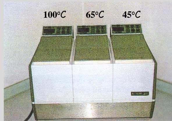
Compartments for liquefying: 100°C, storage: 65°C and tempering the material in a tray at 45°C
