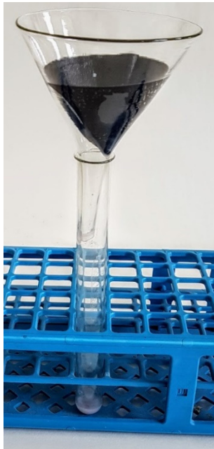
Fig. 4: Filter assembly with a charcoal filter.
