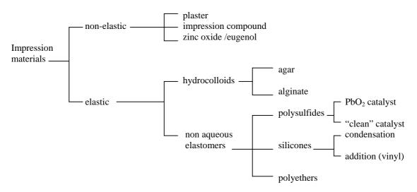
The impression compound consists of about 40 % of natural resins, which make the mixture thermoplastic. Shellac is often used; waxes also make for thermoplastic properties; while stearic acid acts as a lubricant and plasticizer. Fillers and inorganic pigments account for approximately 50 % of the formulation. Diatomaceous earth, soapstone and talc are examples of commonly used fillers.
